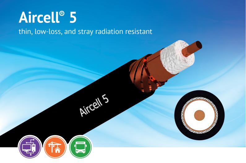
Aircell 5 is a flexible and thin coaxial cable with a 5 mm outer diameter designed for the frequency range from DC to 10 GHz. Its low-loss characteristics in relation to its diameter and compatibility with standard RG 58 connectors make it the preferred choice not only for Wireless LAN applications but also for general RF communications.
