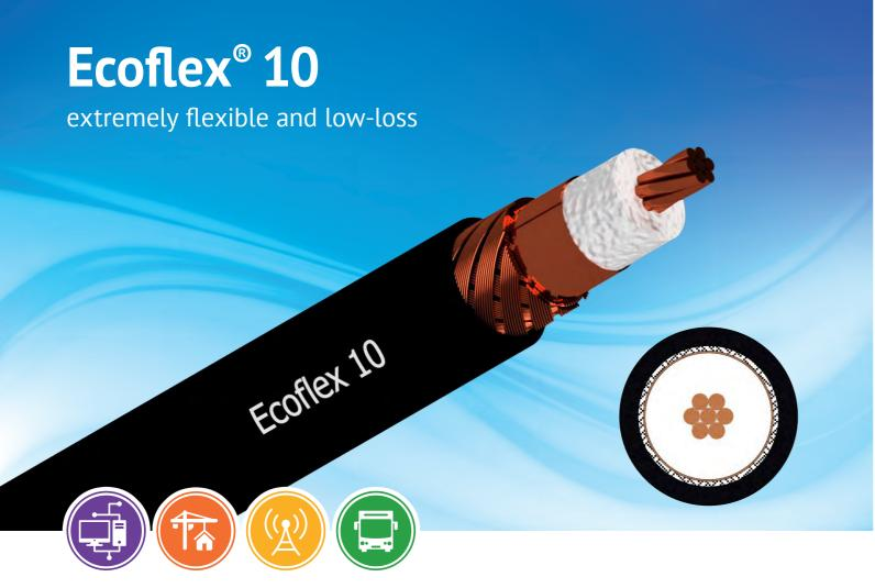
Ecoflex 10 is a flexible and very low-loss 50 ohm coaxial cable designed for the frequency range up to 6 GHz. State-of-the-art production methods and the use of a low attenuation PE-LLC dielectric with a gas content of over 70% enable low attenuation values that set standards for flexible coaxial cables of this size.
