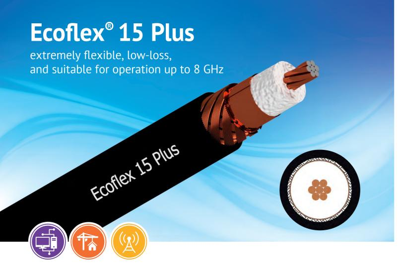
Ecoflex 15 Plus features remarkable electrical and mechanical improvements. The design and use of materials are optimized for minimal loss, an increased maximum frequency by 2 GHz, excellent installation properties, high long-term stability, and, not least, low weight. These optimal physical properties are achieved by using a precision hybrid inner conductor with a micro-welded copper jacket and aluminium core.
