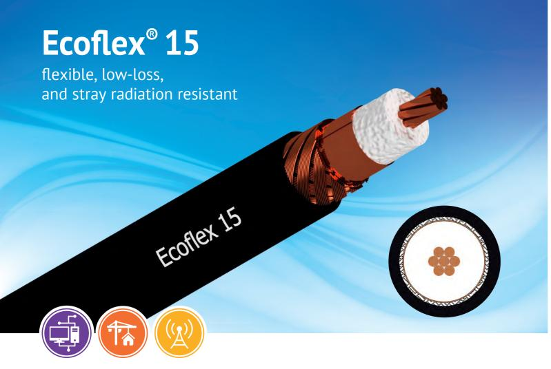
Ecoflex 15 is a flexible and very low-loss 50 ohm coaxial cable for the frequency range up to 6 GHz. State-of-the-art production methods and the use of a low attenuation PE-LLC dielectric with a gas content of over  $70\,\%$  enable low attenuation values.
