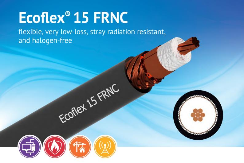
Ecoflex 15 FRNC is a flexible and very low attenuation 50 ohm coaxial cable for the frequency range up to 6 GHz. State-of-the-art production methods and the use of a low attenuation PE-LLC dielectric with a gas content of over 70% enable low attenuation values.
