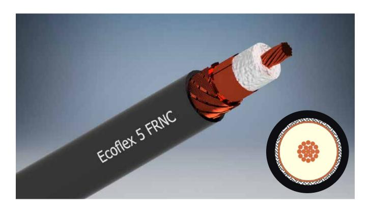
Ecoflex 5 FRNC is a thin and extremely flexible coaxial cable designed for frequencies up to 6 GHz. Due to its low loss in relation to the outer diameter of 5,5 mm and the very small bending radius the cable can be used for numerous RF applications.
