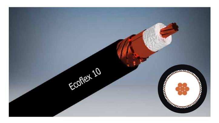
Ecoflex 10 is a flexible, low loss 50 ohm coaxial cable for the frequency range up to 6 GHz. Advanced manufacturing techniques combined with the use of a low loss PE-LLC dielectric with a foaming rate of more than 70% result in very low attenuation values, which set standards among flexible coaxial cables of this dimension.
