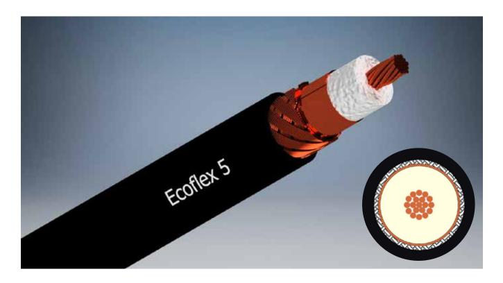
Ecoflex 5 is a thin and extremely flexible coaxial cable designed for frequencies up to 6 GHz. Due to its low loss in relation to the outer diameter of 5,5 mm and the very small bending radius the cable can be used for numerous RF applications.
