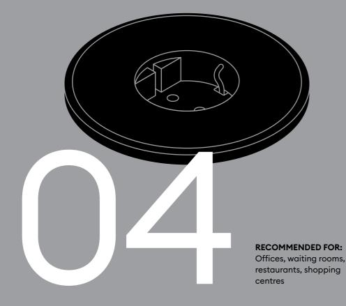
The Iris is a cable grommet with a leaf shutter mechanism which, when the ring is turned, expands or contracts the central opening, adjusting it to a size that will allow cables to pass through. Under the lid inside the bay you can opt for communication connectors, fast USB chargers or power sockets.
