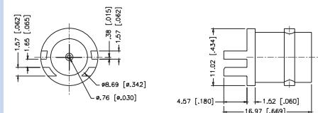
**Bulkhead Vertical P.C. Board Receptacle - End Launch**
