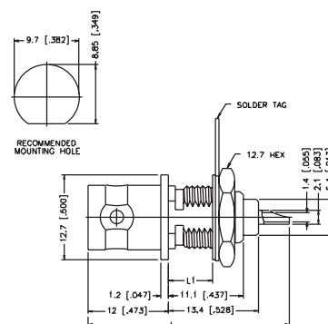
**Bulkhead Receptacle Isolated Jack - Front Mount**
