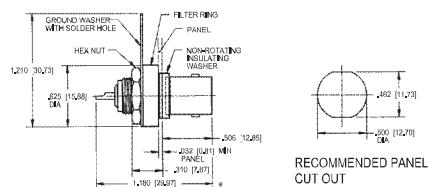
**Bulkhead receptacle BNC Jack - Rear Mount - Crimp**
