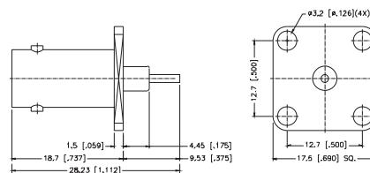
**Panel Receptacle - Exposed Teflon - Gasket Seal**
