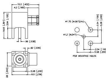
**Edgecard Receptacle for P.C. Board**
