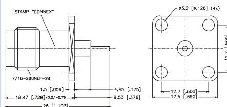
**Panel Receptacle Jack - Extended Teflon Post - Gasket Seal**
