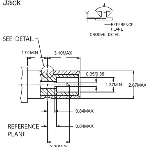
Note: 1. I.D. to meet VSWR and contact resistance when mated with 0.35/0.38 mm dia. Pin.
