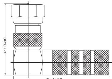
**Bulkhead Crimp and Solder Jack - Flexible and Semi-Rigid Cable**
