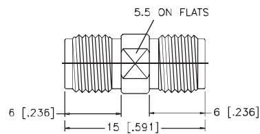
**Jack-to-Jack Adapter - Bulkhead Feedthrough**
