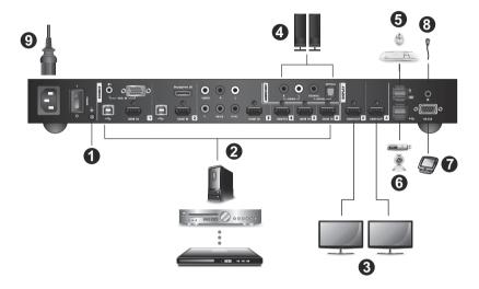
Ground the unit with a grounding wire. Connecting one end of the grounding wire to the grounding terminal, and the other end to a suitable grounded object.
