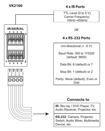
**IR** Connection: Connect a transmitter cable to the IR and Ground ports on the Control Box and install the IR transmitter on or near the device's IR receiving port, as shown on page 28.
