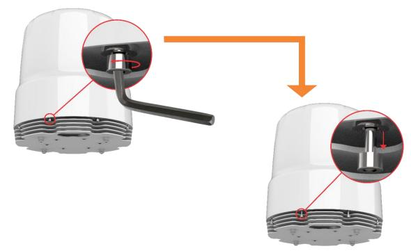
Using the 5mm Allen/hex key in the provided tool kit and unscrew the M8 cap screws. The Cap screws are captive screws and only need to be unscrewed till it drops loose into the cavity below. Continue to the next step.
