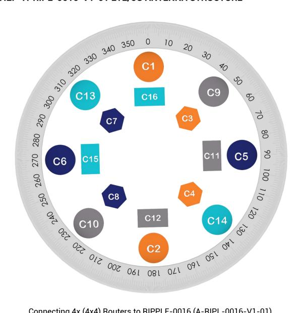
Connecting 4x (4x4) Routers to RIPPLE-0016 (A-RIPL-0016-V1-01)
