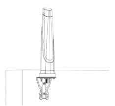
Antenna Configuration 3 Surface mount with adhesive disc Use adhesive disc as template for drilling a cable hole
