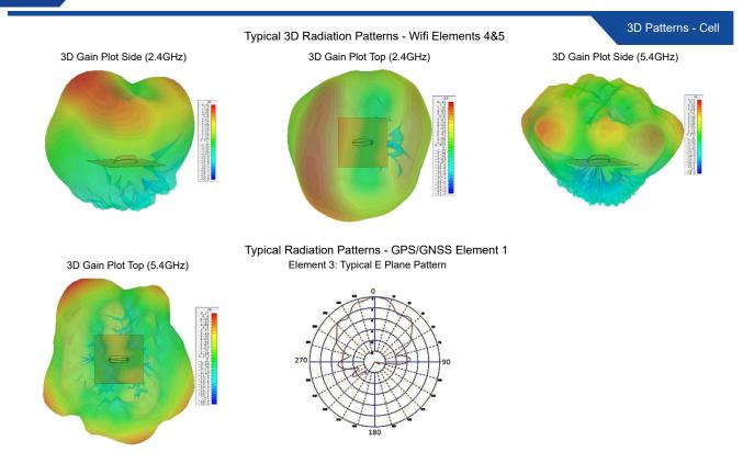
\*3D radiation patterns simulated in CST Microwave Studio on a 600x600mm (2' X2') ground plane with both elements fed together.
