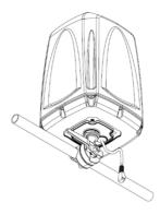
**Note:** The installer should ensure that the BRKT-38 cable entry hole is adequately waterproofed to maintain the CPE's IP rating. Additionally, should the thread of the marine mount bracket protrude too far into the CPE, make use of the locking nuts to raise the CPE base on it.
