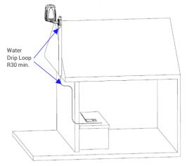
Note: The water drip loop is for preventing water from running down from the CPE along the cable into the house and possibly the PC or router.
