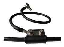
The GC-10 grounding clamp was developed for equipotential bonding on 10 mm coax cables such as ECOFLEX 10, Aircom Premium etc. This eliminates potential differences (voltages) between the coax cable and the earth potential. Especially during thunderstorms, charging can occur on the antenna or on the coax cable. This charge is removed with the earthing clamp and the connected device is protected. A grounding clamp is not a replacement for lightning protection.
