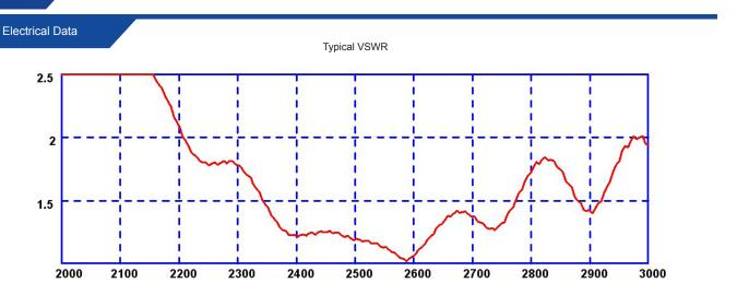
\*VSWR mounted on glass sheet with 3m (10') of RG174 cable
