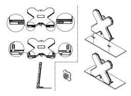
2 Installing using adhesive pad
