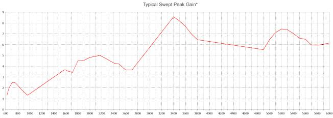
\* Swept peak gain simulated in CST Microwave Studio without cable loss.
