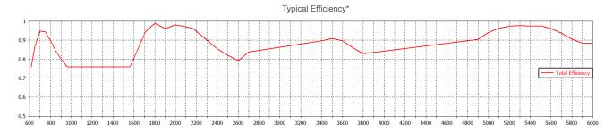
\*Element efficiency simulated in CST Microwave Studio without cable loss.
