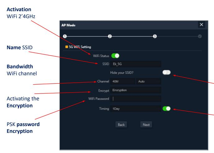
The configuration of the 5GHz radio is analogous to that of 2'4GHz, depending also on the active advanced configuration.
