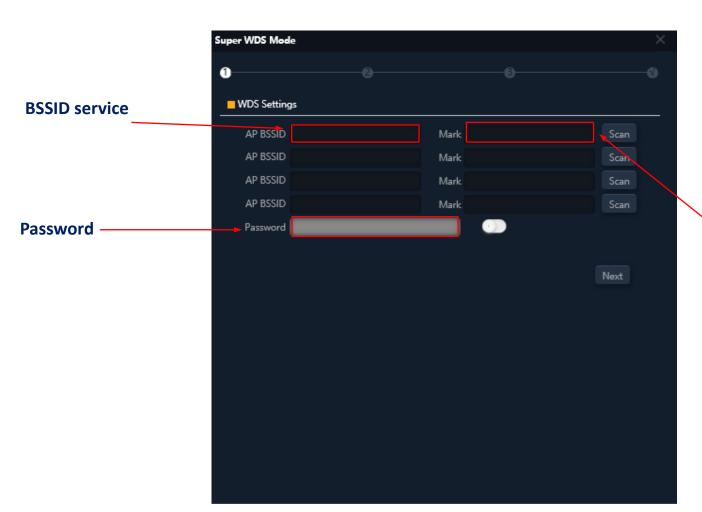
In **SUPER WDS** mode, a point-to-point connection is established with the selected emitter.
