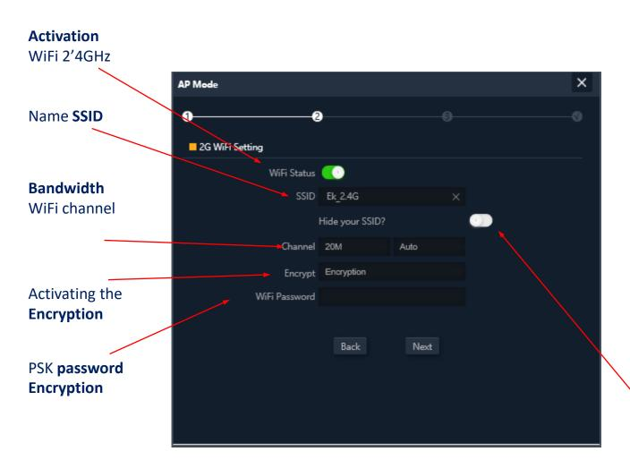
The **setup wizard** allows you to configure the basic parameters of the two WiFi radios. The parameters offered as an option depend on the active advanced settings (WiFi section).
