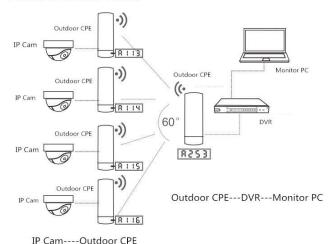
The CPE operation mode is configured by selecting the WDS option in the wizard, thus being able to configure point-to-point or multipoint connections (with a maximum of up to 4 terminals or CPEs)
