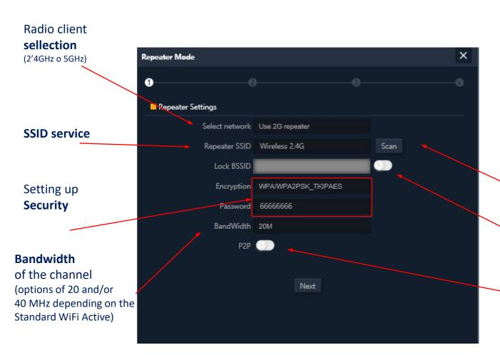
In **WISP** and **Repeater** modes the Internet output is established with a WiFi connection to an existing service (service SSID). A radius of the **APs** is configured as a client and thus establishes the link to output user traffic.
