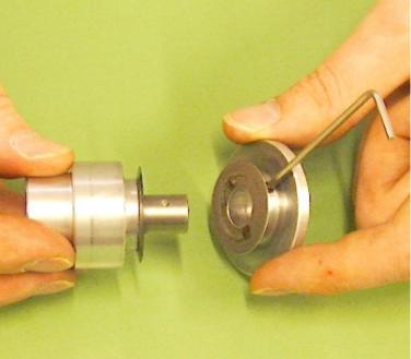
Loosen the fastening screws of the knife blades and remove blades.
