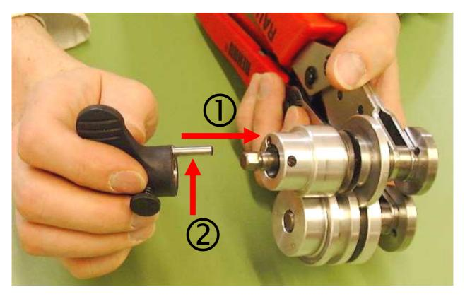
The butterfly handle can be plugged on the axis completely, when the driver pin locks into the driver tooth system inside the cutting weel.
