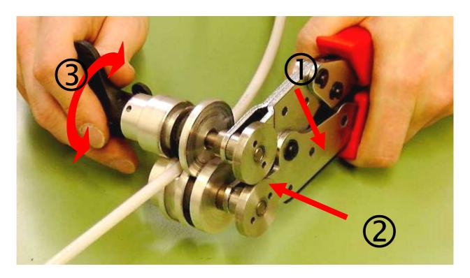
By continuous turning the handle the buffer tube can be opened up to the required length.
