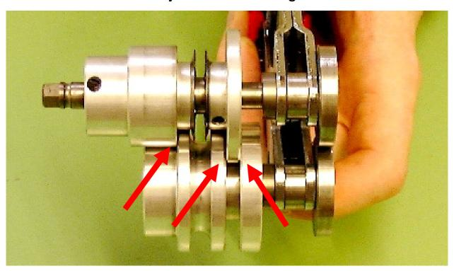
The adjustment is fixed while inserting (1) the driver pin (2) of the butterfly handle.
