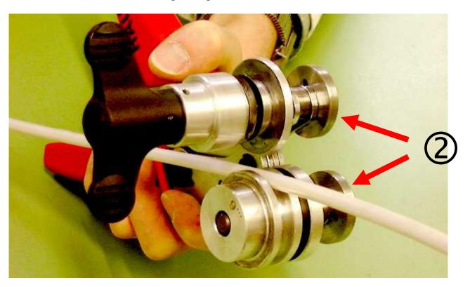
Close the tool <u>slowly</u> (1) until the guide axis roller touches the cutting axis roller (2). <u>Simultaneously</u> turn the butterfly handle backwards and forwards (3), to enable the knifes to cut gently into the buffer tube. This prevents the thin knife blades from damage.
