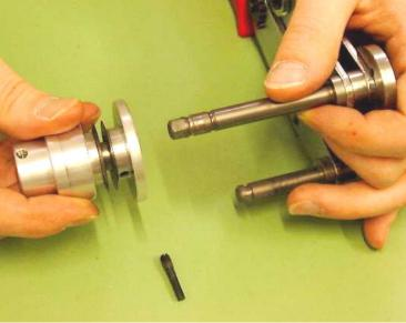
During assembly the tapered screw is fixed with care. The cutting weel must be free from play but easily turneable onto the axis!
