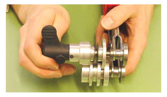
The cutting width is fixed now for the cutting of the buffer tube.
