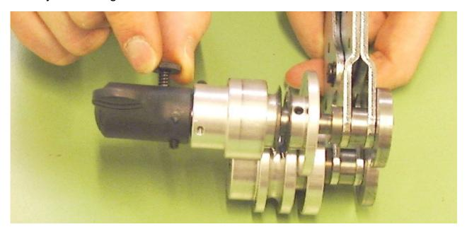
The tool with fixed cutting weel then is pulled over the flexible buffer tube.
